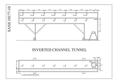
Figure 3.1.1: Diagram of SANS 10177-10 inverted channel testing facility
