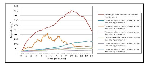
Figure 4.1.2: Temperatures recorded during the test on 100 mm thickness Fabufill ceiling insulation material
